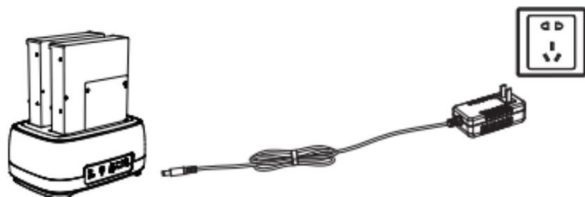
2. Insert the disk that needs to be cloned into the source bay and the disk waits to be cloned into the target bay.
